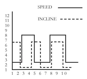
The Weight Loss Program is designed to alternate between the programmed speed and incline. The program will alternate between: 1) the full programmed incline and half the programmed speed, to 2) zero incline and the maximum programmed speed.
